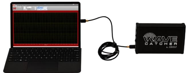
**Figure 3:** Notebook Computer Connected to ADC
