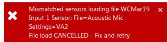
**Figure 45:** Error Message When Mismatched Sensors Are Being Used
