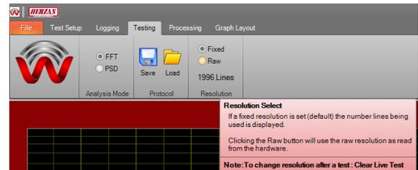
**Figure 39:** Selecting Desired Resolution Option
