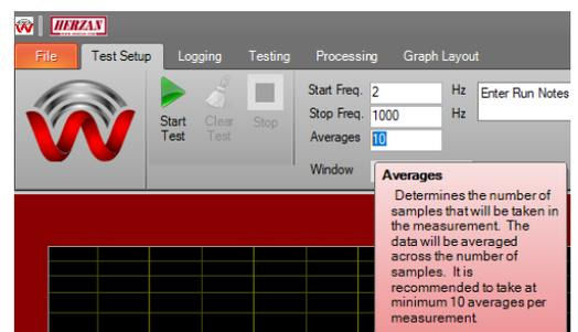
**Figure 18:** Setting the Number of Averages Taken Per Measurement
