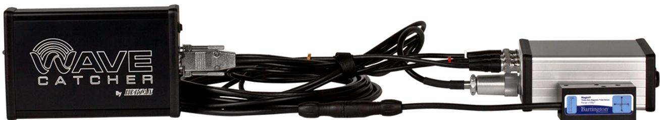
Figure 9: Bartington EMI Sensor Connected to the ADC
