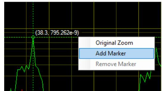
**Figure 28:** Selecting A Point On the Graph to Set As A Marker
